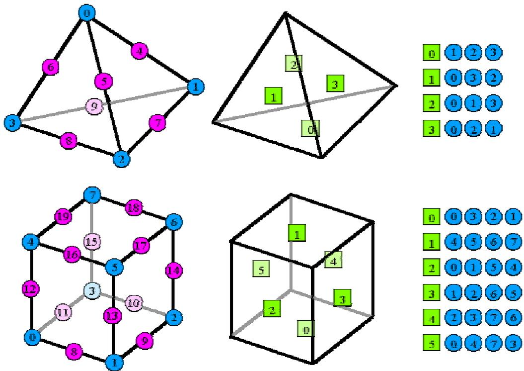
Fig. Basic Elements (the node numbers are shown in circles, and the surface numbers are shown in squares)
